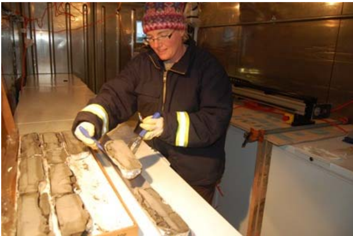
Figure 104: Step 5: Core sections were carefully placed into one-third liners (see "Potential Artifacts," above)
