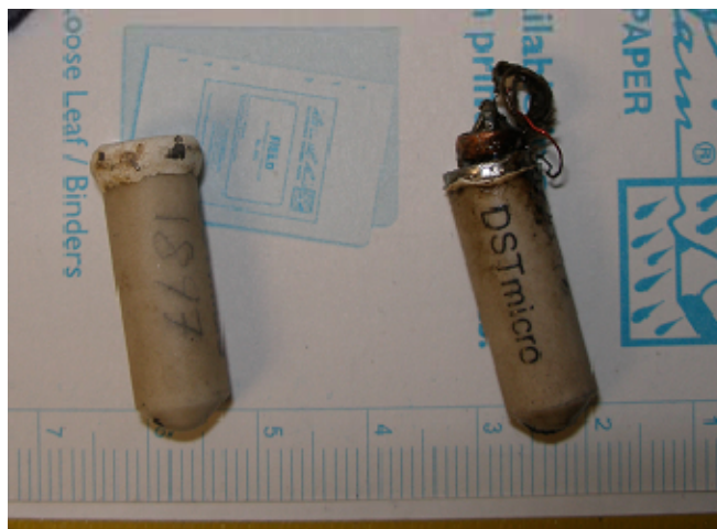
Figure 61: DSTmicro capsule data logger used to record time, temperature, and pressure during coring and during MDT logging operations (data logger on right was destroyed during operations outside the pressure rating of logger)
