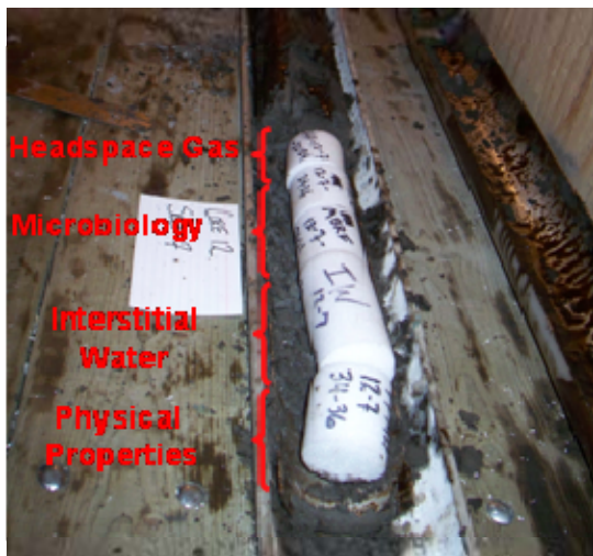
Figure 81: Foam inserts mark where core was subsampled for headspace gas, microbiology, interstitial water and physical properties (appendix A of R18 contains onsite descriptions)
