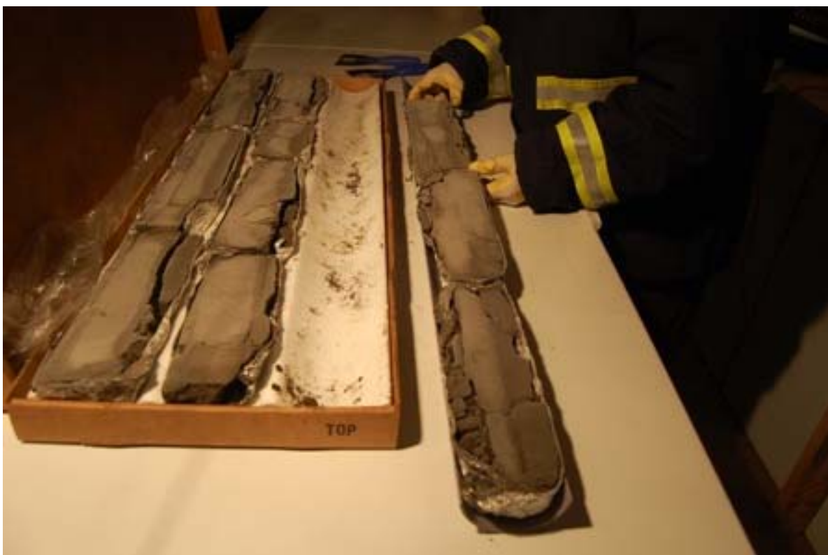
Figure 105: Step 6: Complete placement of core sections into one-third liners
