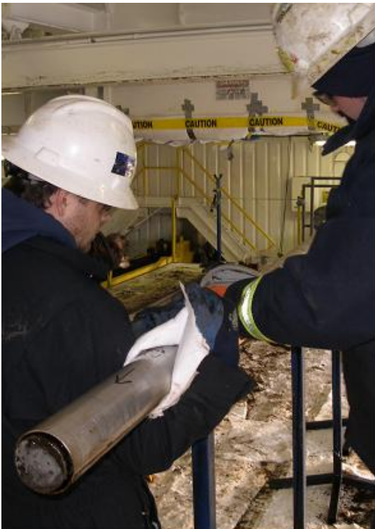
Figure 77: Core inner barrel cutting into 3 foot segments in pipeshed with core end visible in lower left side of photo
