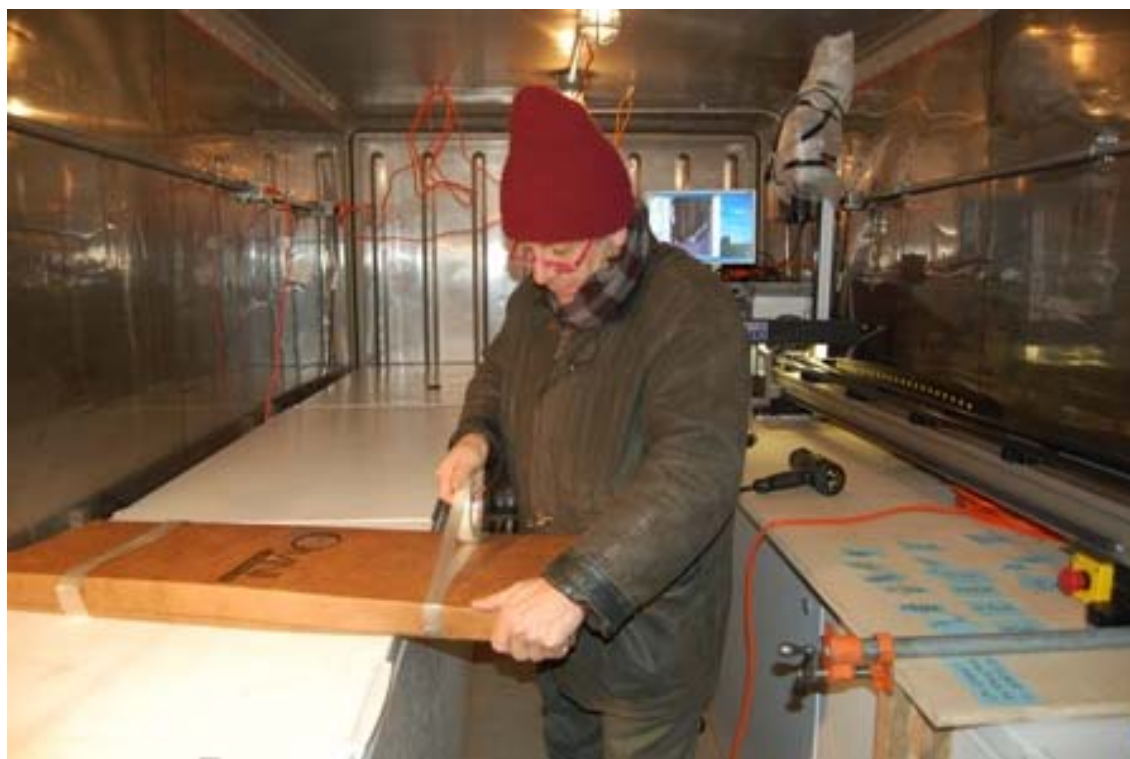
Figure 114: Step 15: Core storage boxes were closed with strapping tape wrapped around ends
