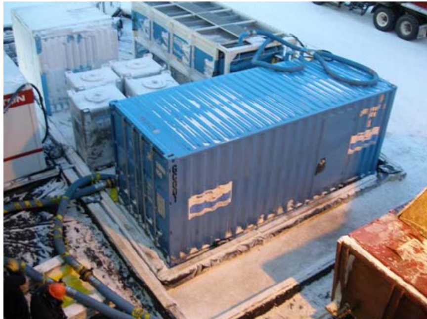
Figure 54: DrillCool, Inc. Heat Exchange Mud Chilling Unit at Mt Elbert-01
