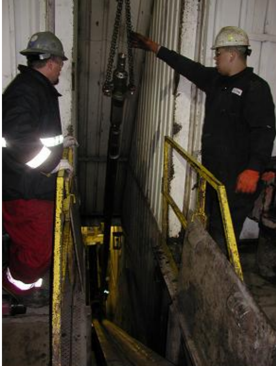
Figure 75: Core barrel being lowered from rig floor to pipeshed via V-door
