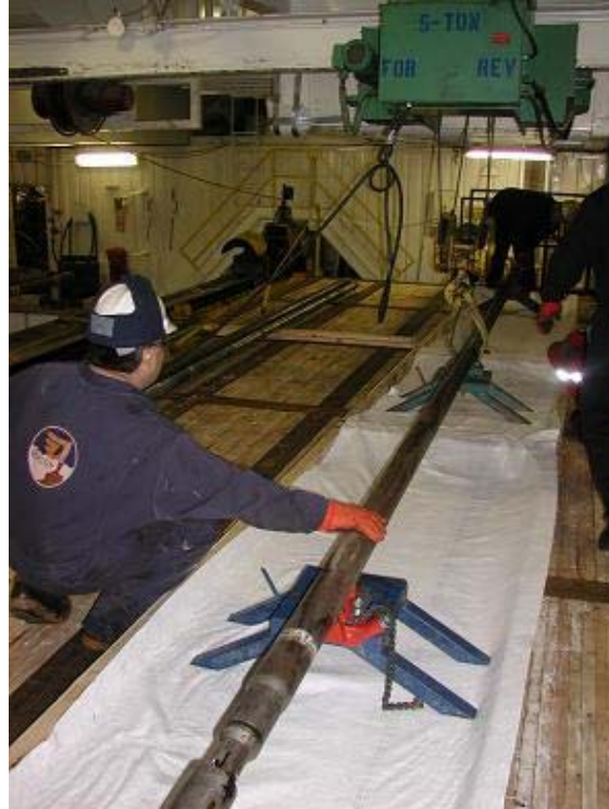
Figure 76: Core barrel inner liner separation in cold pipeshed processing area; rig mats placed on pipe racks provided working surface
