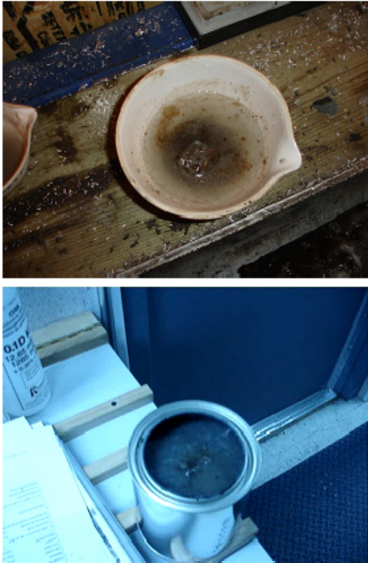
Figure 83: Gas hydrate-bearing samples in water bubble with gas escape during gas dissociation onsite testing for gas hydrate presence in core samples
