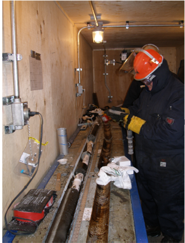
Figure 84: Gas hydrate-bearing sediment placed in syringe to monitor gas escape from gas hydrate dissociation in hydrate-bearing core samples during onsite analyses
