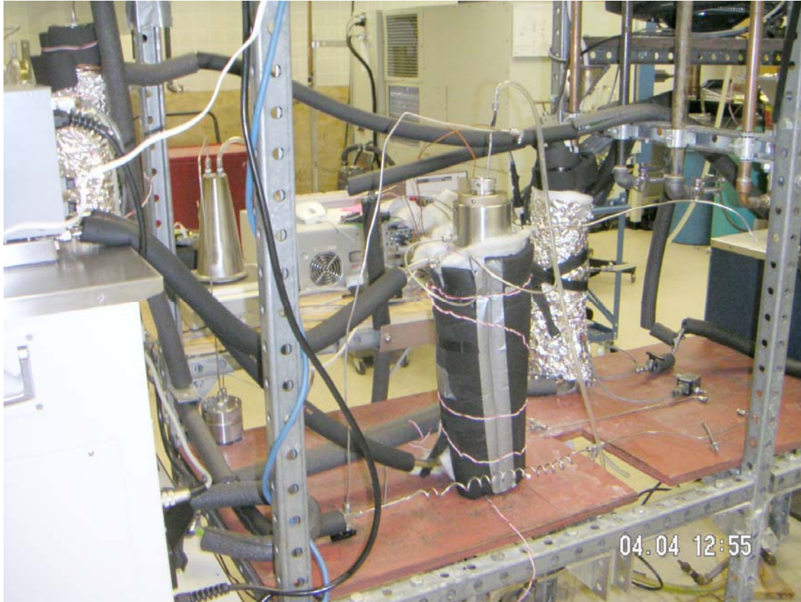
Figure 24: The experimental set-up constructed for forming gas hydrate and measuring relative permeability (April 2004)
