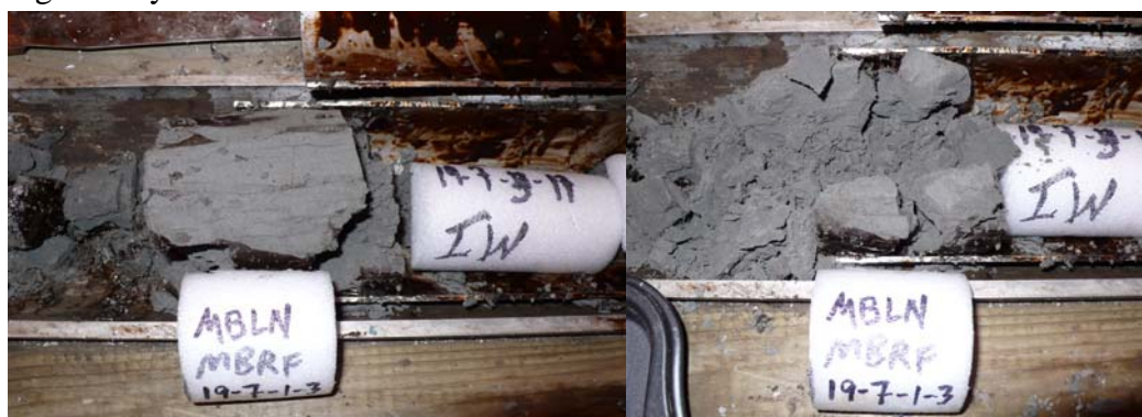
Figure 91: Photo of core run #19, section 7, inches 1-3 after shaving the drilling fluids away from the surface and before scooping the inner portions of the core for microbiological analysis (left) and after scooping the inner portions (right).
