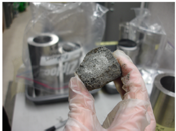
Figure 86: Cleaner innermost portion of core prior to placement into drill-press to remove formation water for later laboratory analyses
