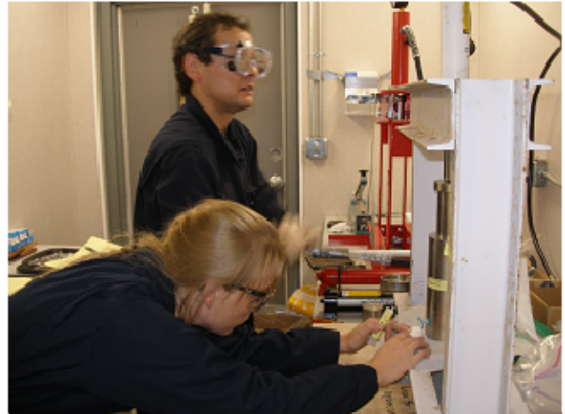
Figure 88: Warren Agena (USGS) and Kelly Rose (USDOE) work the drill-press to obtain interstitial water for later analyses
