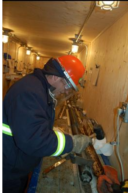
Figure 80: Robert Hunter (BPXA consultant) subsamples gas hydrate-bearing core in core processing “cold” trailer, February 2007
