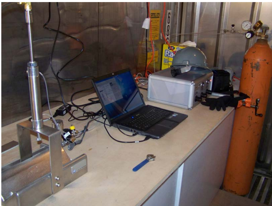
Figure 121: UAF Minipermeameter feasibility test setup in gas hydrate core storage unit (March 2008)
