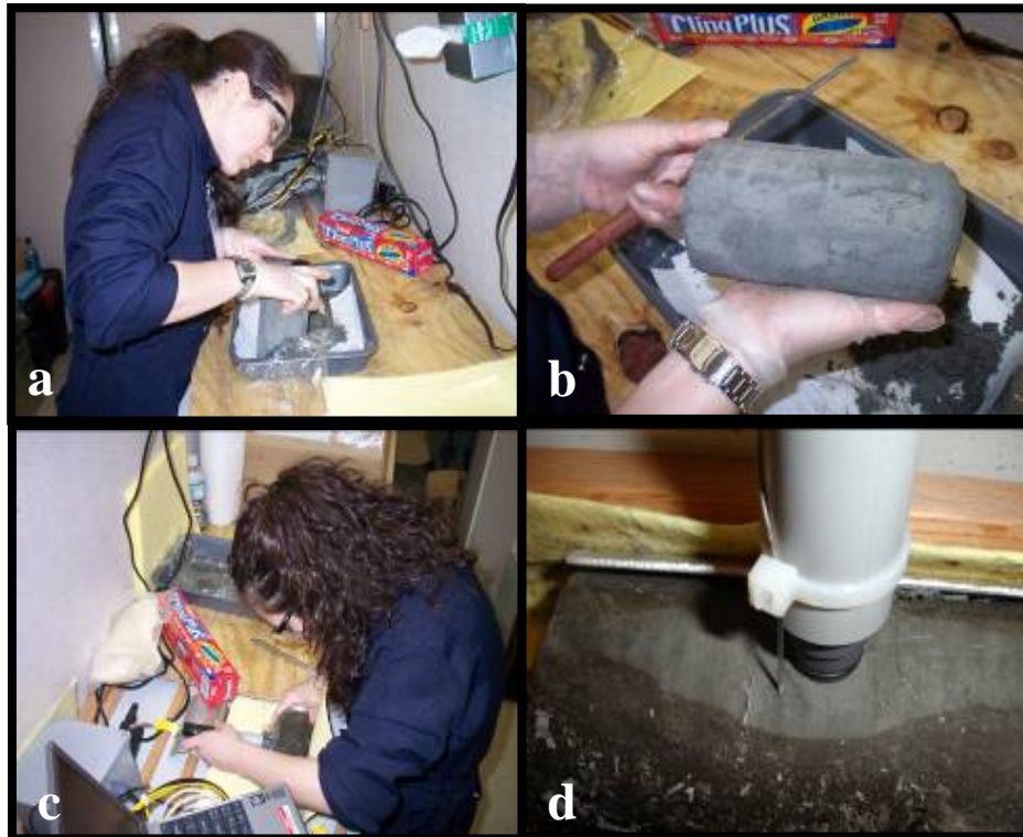
Figure 94: Sample preparation and thermal properties measurement. Drilling mud was removed prior to measurements (a and b). For time critical measurements on gas hydrate-bearing sediments, only a portion of the drilling mud was removed for measurements (c and d).
