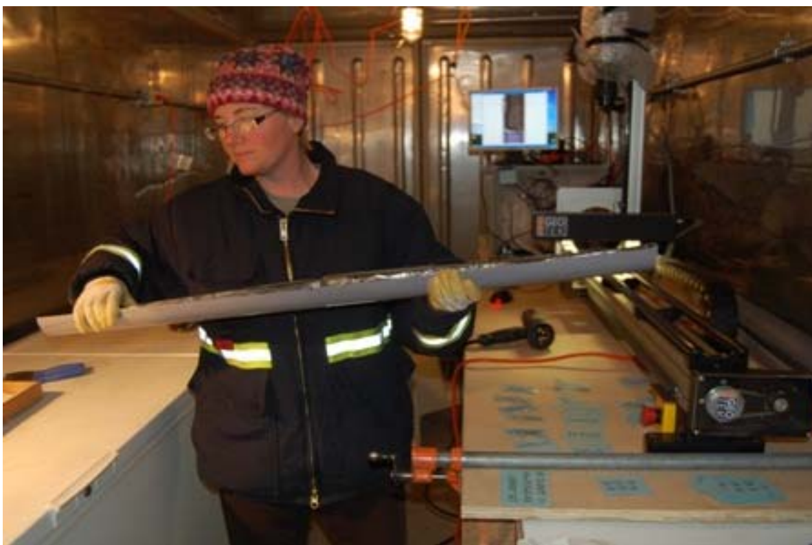
Figure 109: Step 10: Core sections within the liner were removed from the camera track
