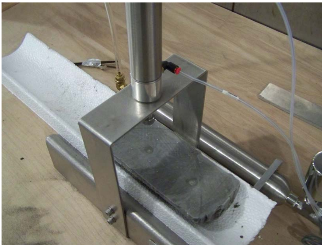
Figure 122: Mt Elbert core in minipermeameter apparatus during feasibility test (March 2008)
