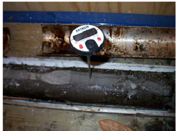
Figure 82: Temperature probe test used to show decreased temperature with time during gas hydrate dissociation in hydrate-bearing core samples during onsite subsampling
