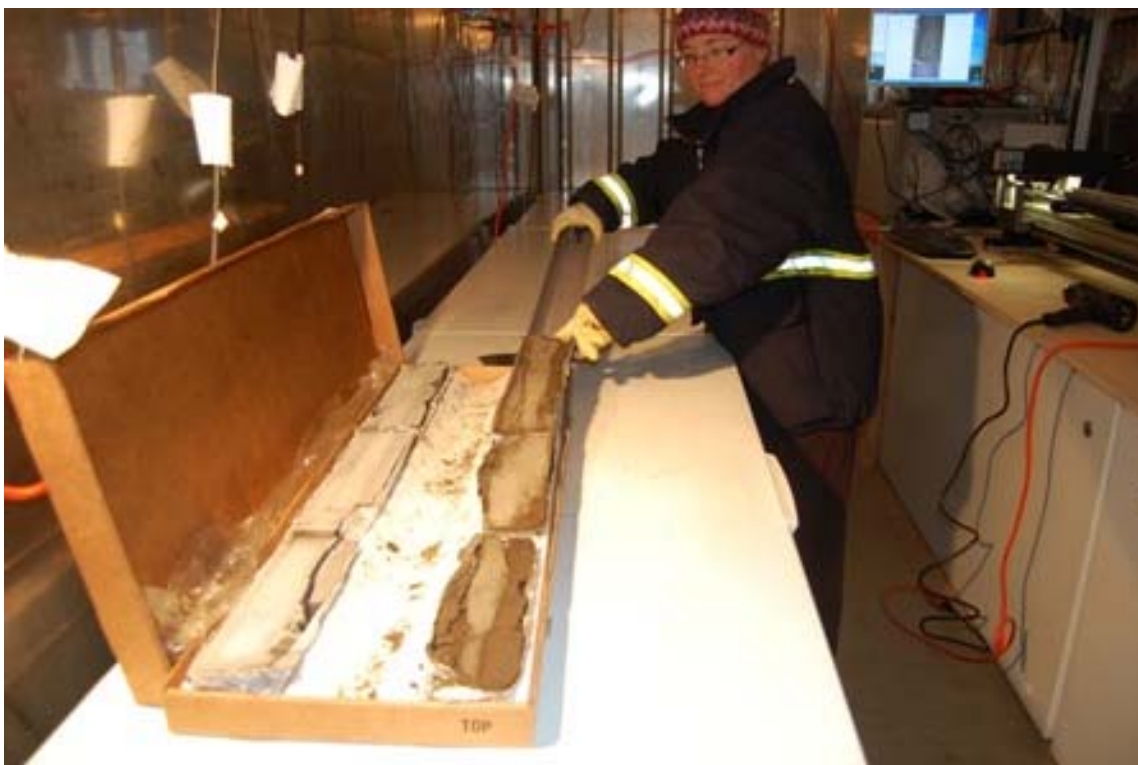
Figure 111: Step 12: The core sections were gently removed from the track in the liner and placed back into the core storage box
