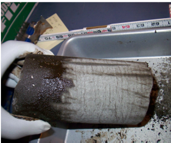
Figure 85: Whole core sample is scraped to remove oil-based drilling mud contamination
