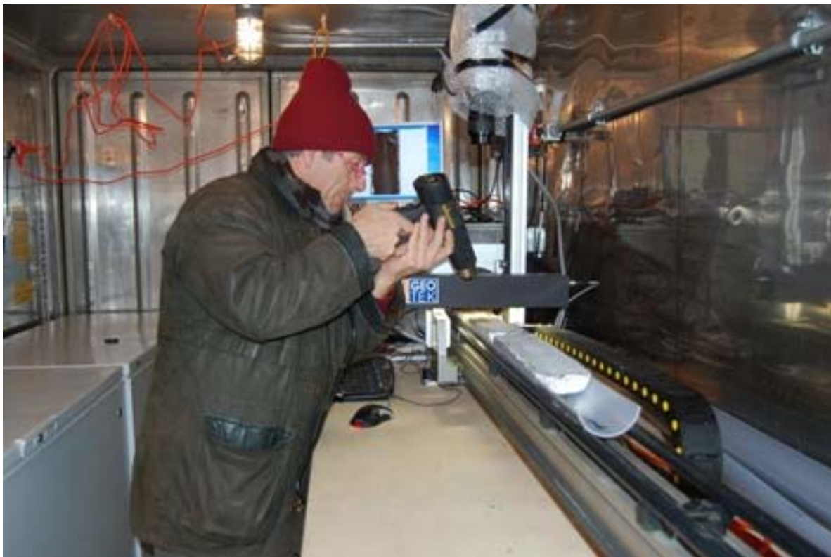
Figure 108: Step 9: Core surfaces were heated using a heat gun to melt surface frost, typically resulting in a wet surface when imaged (see "Potential Artifacts," above)
