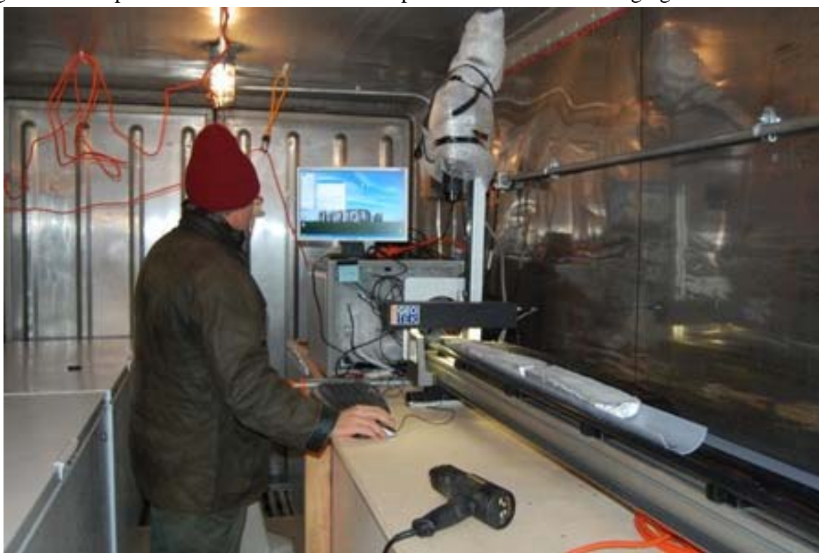
Figure 107: Step 8: Cores were scanned at a resolution of 200 pixels per centimeter at a single set of lighting and aperture conditions, and the camera was consistently calibrated with an 18% grey card so that each image is comparable with every other image
