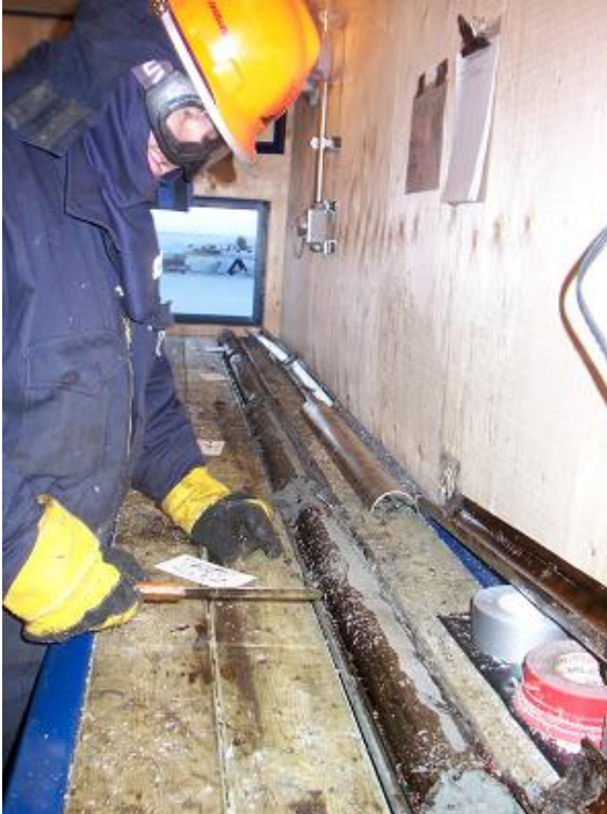
Figure 79: Dr. Timothy Collett (USGS) scrapes and describes gas hydrate-bearing core in core processing “cold” trailer, February 2007
